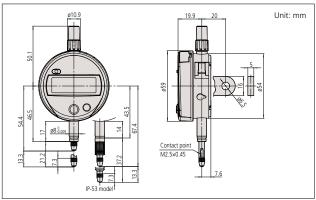
Note 1: Dimensions of the inch (ANSI/ AGD Type) dial indicator partly differ from those of the metric (ISO/JIS Type) indicator. Note 2: Inch (ANSI/AGD Type) dial indicators are provided with a stem of 3/8" dia. and #4-48UNF thread mount for the contact point.
