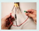
GREEN LED means wiring is properly identified.
