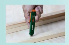
Take quick Moisture level reference on wood and building materials (such as brick and concrete) with this convenient portable Moisture Pen. Easy-to-read dual color LED indication with 10 ranges of %WME moisture level. Ideal for building restoration applications such as detecting water leakages inside walls, ceilings, and floors.
