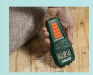
Take quick moisture level reference measurements on wood and building materials with this convenient compact-sized pin-type Moisture Meter. Easy-to-operate with display icons that indicate the levels of moisture content plus audible alert feature. Ideal for building restoration projects and applications where moisture detection on floors and under carpets is critical. A must-have tool for analyzing the after-effects of water leakage behind walls and in ceilings.
