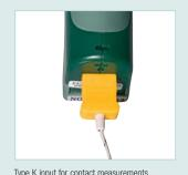
Type K input for contact measurements
