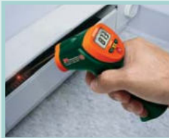
Test for temperature in heating systems
