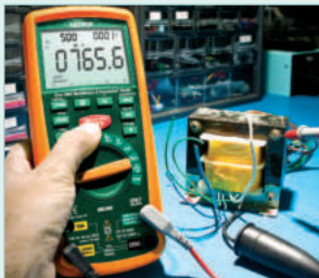
Measure the insulation resistance of transformer windings
