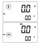
• To save a 1-point procedure, press CAL. The instrument will memorize the zero calibration data and return to measurement mode.
