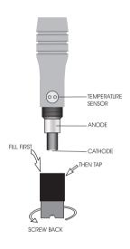
If any deposit scales the sensors, gently brush the sensor surface with the supplied scouring pad, while paying attention to not damage the plastic body.
